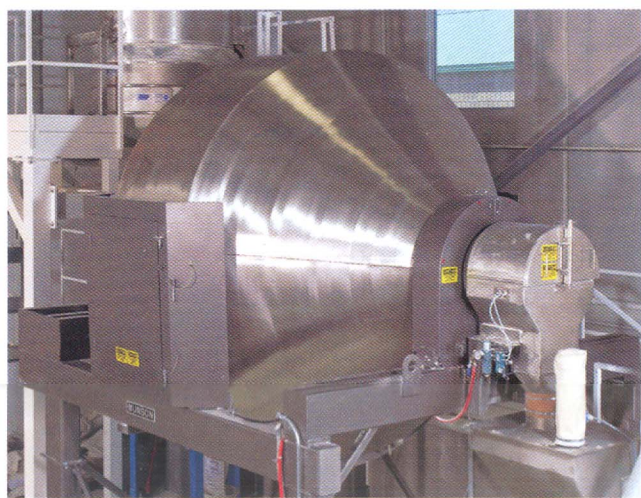
Upon discharge, the rotary batch mixer evacuates completely with little or no residual, allowing, fast thorough cleaning between batches.
